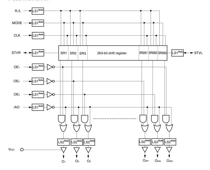
Note LS1: shifts CMOS level and internal level, LS2: shifts interval level and output level (VDD2 to VEE2).
