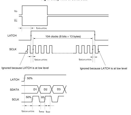
Fig 1. Delay Time of Serial Data
