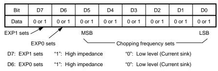
The chopping frequency is set to 0 kHz and to a value in the range of 35.71 kHz to 225 kHz (4.5 MHz clock input). Refer to table 1 (4 page).
