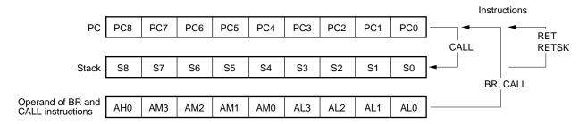
In Fig. 2-1, AHn, AMn, and ALn  $(0 \le n \le 3)$  indicate bit positions in a 16-bit instruction as follows:
