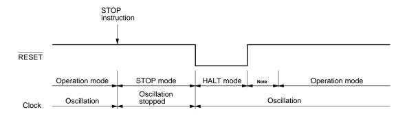
As soon as the RESET input makes a transition from high to low in the STOP mode, the system clock starts generating clock pulses.
