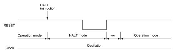
When the  $\overline{\text{RESET}}$  signal is applied to release the HALT mode, the  $\overline{\text{RESET}}$  input makes a transition from low to high, then an operation mode is entered.
