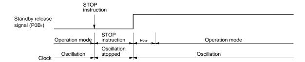
**Note** The HALT mode remains effective in this period, waiting for the generation of clock pulses to settle. An operation starts after eight clock pulses on the OSC<sub>0</sub> pin are counted.
