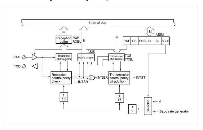
Figure 8-1. Block Diagram of Asynchronous Serial Interface
