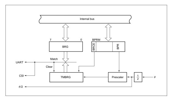
Figure 8-3. Block Diagram
