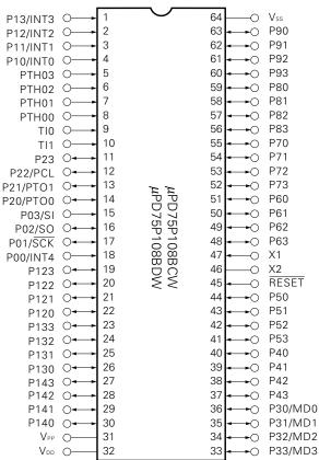
64-pin plastic QFP (14  $\times$  20 mm, 1.0 mm pitch)
