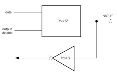
This is an input/output circuit made up of a Type D push-pull output and Type B Schmitt-triggered input.
