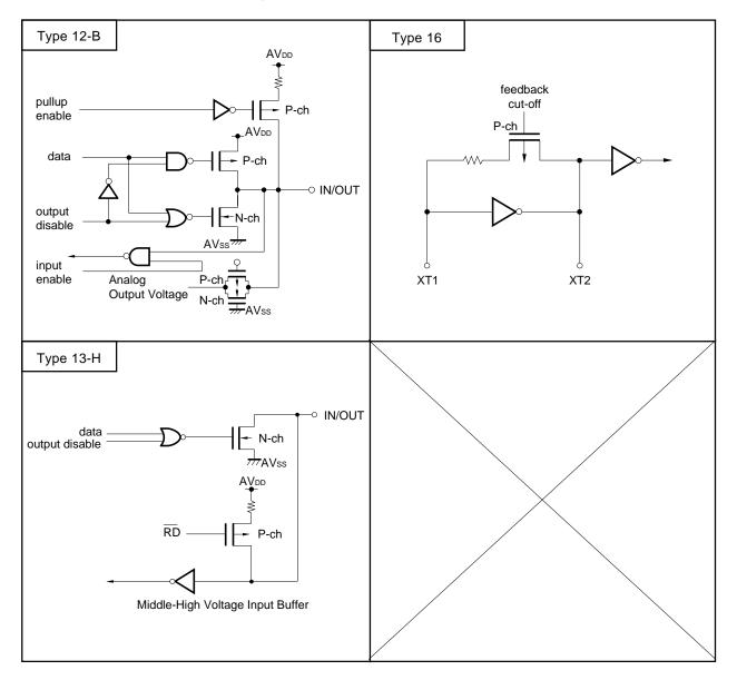
Figure 2-1. Pin Input/Output Circuits (2/2)
