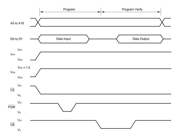
Figure 5-4. Byte Program Mode Timing
