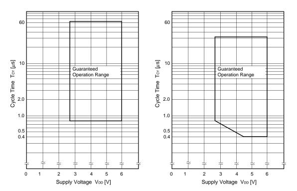
Tcy vs VDD (Main System Clock, fxx = fx)
