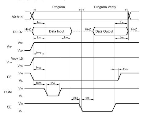
Cautions 1. VDD should be applied before VPP, and removed after VPP.
