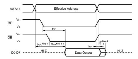
Notes 1. If you want to read within the range of tacc, make the  $\overline{OE}$  input delay time from the fall of  $\overline{CE}$  a maximum of tacc-
