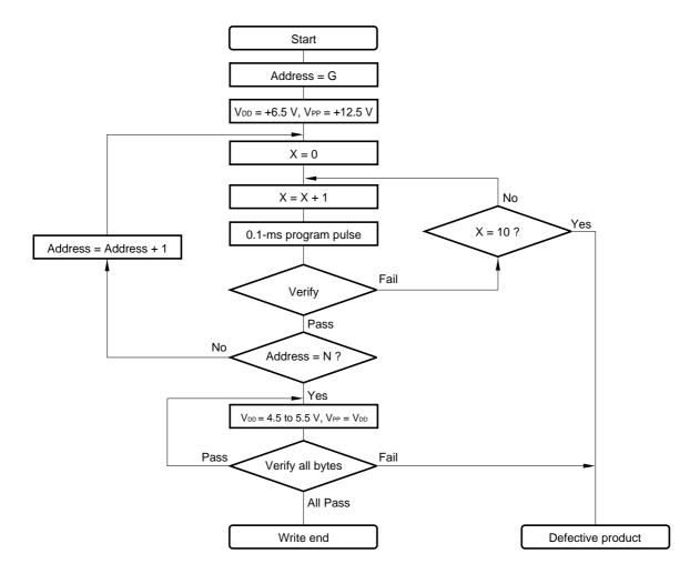
Figure 4-3. Byte Program Mode Flow Chart
