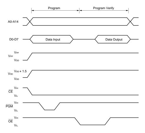
Figure 4-4. Byte Program Mode Timing
