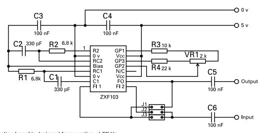
The evaluation board is designed for operation at 70kHz.
