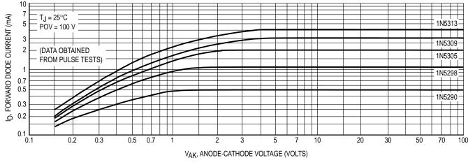
**Figure 3. Typical Forward Characteristics**
