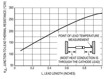
Figure 2. Typical Thermal Resistance
