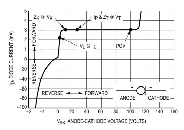
Figure 1. Typical Current Regulator **Characteristics**
