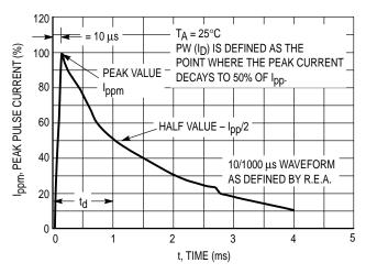
Figure 4. Pulse Waveform 10/1000
