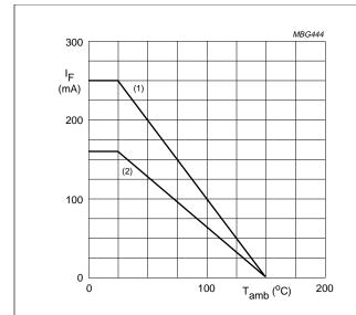
Device mounted on an FR4 printed-circuit board.
