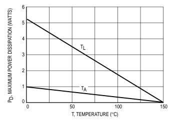
Figure 5. Steady State Power Derating
