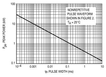
Figure 1. Pulse Rating Curve
