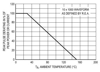
Figure 3. Pulse Derating Curve
