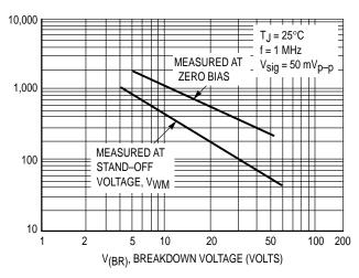
**Figure 4. Typical Junction Capacitance**
