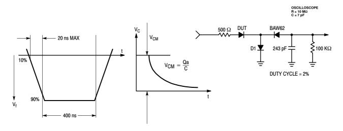
Figure 2. Stored Charge Equivalent Test Circuit
