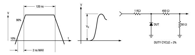
Figure 3. Forward Recovery Voltage Equivalent Test Circuit
