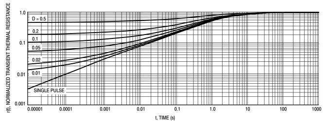
Figure 7. Normalized Thermal Response
