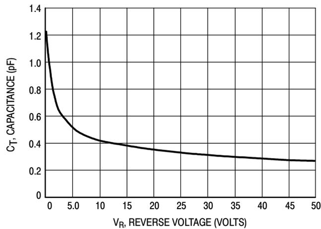
Figure 3. Typical Capacitance
