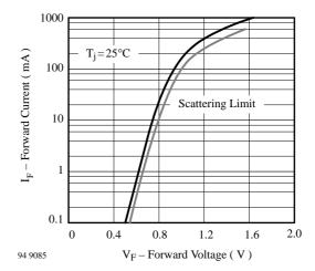
Figure 2. Forward Current vs. Forward Voltage
