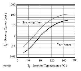
Figure 1. Reverse Current vs. Junction Temperature
