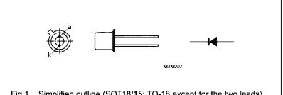
Fig.1 Simplified outline (SOT18/15; TO-18 except for the two leads) and symbol.
