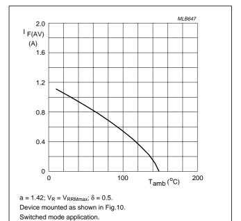
Fig.3 Maximum permissible average forward current as a function of ambient temperature (including losses due to reverse leakage).
