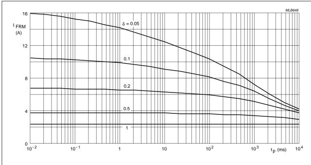
$T_{tp} = 50^{\circ}C; R_{th j-tp} = 25 \text{ K/W}.$
