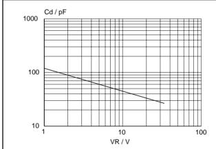
Fig.6. Typical junction capacitance per diode;  $C_d = f(V_R)$ ; f = 1 MHz;  $T_j = 25$ °C to 125°C.
