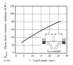
Figure 2. Thermal Resistance vs. Lead Length
