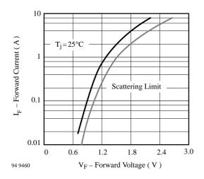
Figure 6. Forward Current vs. Forward Voltage
