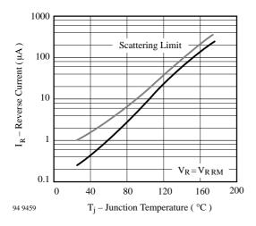
Figure 5. Reverse Current vs. Junction Temperature
