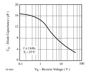
Figure 7. Diode Capacitance vs. Reverse Voltage
