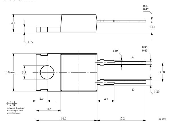
Cathode connected with metallic surface , Plastic Case DO 220 , Weight max.: 2.5  $\ensuremath{g}$
