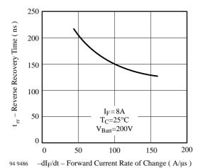
Figure 9. Reverse Recovery Time vs. Forward Current Rate of Change
