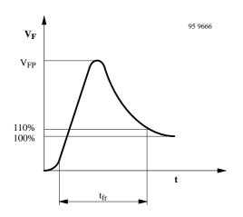
Figure 1. Turn on transient peak voltage
