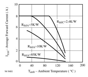
Figure 5. Average Forward Current vs. Ambient Temperature
