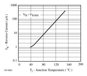
Figure 4. Reverse Current vs. Junction Temperature
