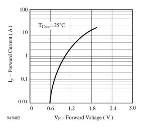
Figure 6. Forward Current vs. Forward Voltage
