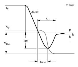
Figure 3. Turn off switching characteristic
