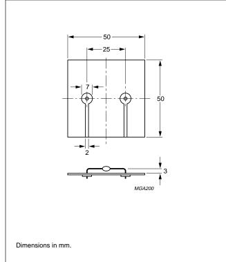
Fig.12 Device mounted on a printed-circuit board.
