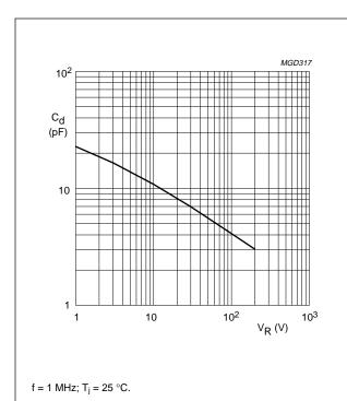
Fig.11 Diode capacitance as a function of reverse voltage; typical values.
