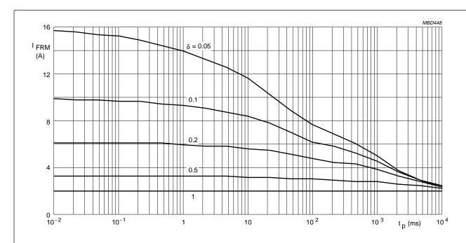
$T_{tp} = 65^{\circ}C$ ;  $R_{th j-tp} = 46$  K/W.
