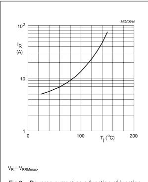
Fig.8 Reverse current as a function of junction temperature; maximum values.
