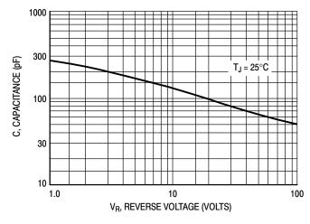
Figure 7. Typical Capacitance, Per Leg
