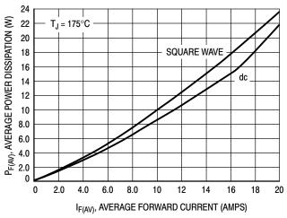
Figure 6. Power Dissipation, Per Leg
