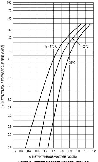
Figure 1. Typical Forward Voltage, Per Leg
