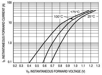
Figure 2. Maximum Forward Voltage
