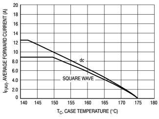
Figure 4. Current Derating, Case, Per Leg
