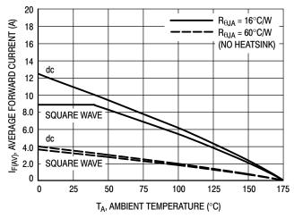
Figure 5. Current Derating, Ambient, Per Leg
