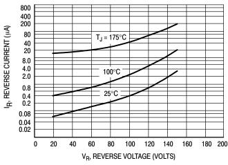
Figure 3. Typical Reverse Current, Per Leg\*
