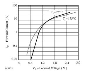
Figure 6. Forward Current vs. Forward Voltage
