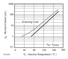
Figure 5. Reverse Current vs. Junction Temperature
