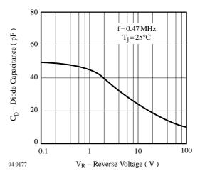
Figure 7. Diode Capacitance vs. Reverse Voltage
