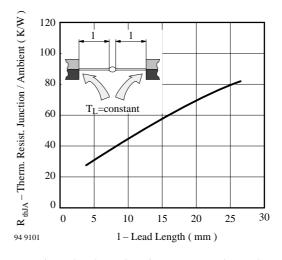
Figure 2. Thermal Resistance vs. Lead Length
