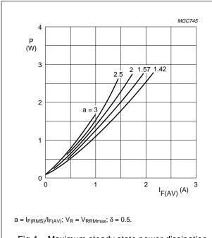
Fig.4 Maximum steady state power dissipation (forward plus leakage current losses, excluding switching losses) as a function of average forward current.
