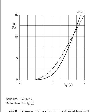
Fig.6 Forward current as a function of forward voltage; maximum values.
