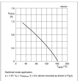
Maximum permissible average forward current as a function of ambient temperature (including losses due to reverse leakage).
