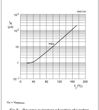
Fig.7 Reverse current as a function of junction temperature; maximum values.
