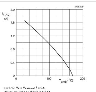
Device mounted as shown in Fig.11. Switched mode application.
