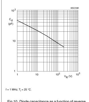
Fig.10 Diode capacitance as a function of reverse voltage; typical values.
