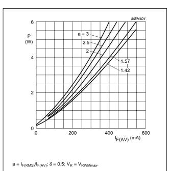
Maximum steady state power dissipation (forward plus leakage losses) as a function of average forward current.
