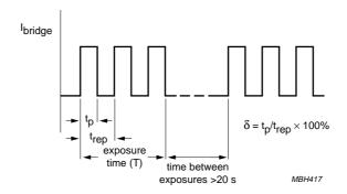
Fig.10 Maximum current through a 3-phase bridge rectifier versus pulse duration; exposure time T = 3 s;  $T_{oil}$  = 50 °C.
