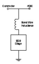
Figure 3. Standard ESD Protection Model
