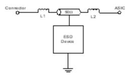
Figure 4. CM1234 PicoGuard XS ESD Protection Model
