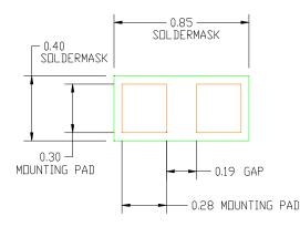
Figure 6. Recommended Mounting Pattern
