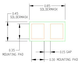
Figure 7. Maximum Recommended Mounting
