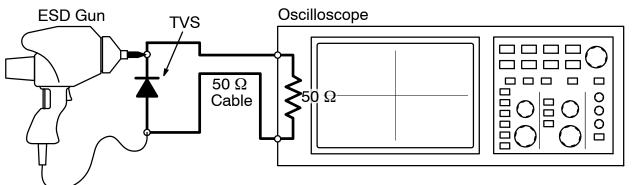
Figure 4. Diagram of ESD Test Setup
