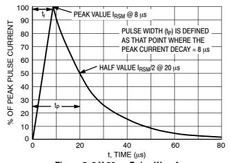
Figure 5. 8 X 20 μs Pulse Waveform
