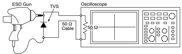
Figure 4. Diagram of ESD Test Setup
