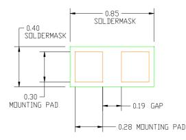
Figure 6. Recommended Mounting Pattern
