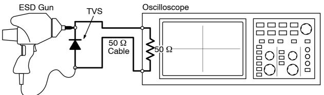
Figure 4. Diagram of ESD Test Setup
