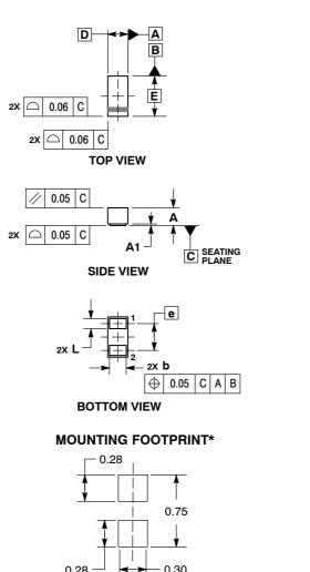
DIMENSIONS: MILLIMETERS See Application Note AND8398/D for more mounting details
