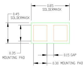
Figure 7. Maximum Recommended Mounting
