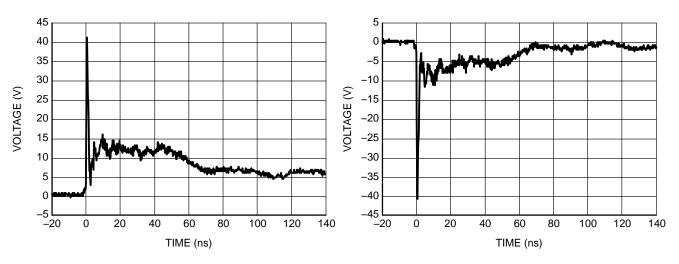
Figure 2. IEC61000-4-2 +8 kV Contact ESD Clamping Voltage
