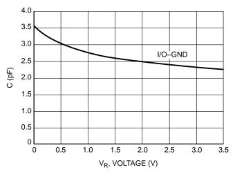
Figure 6. CV Characteristics
