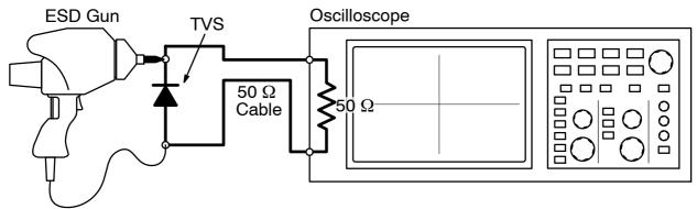
Figure 4. Diagram of ESD Test Setup
