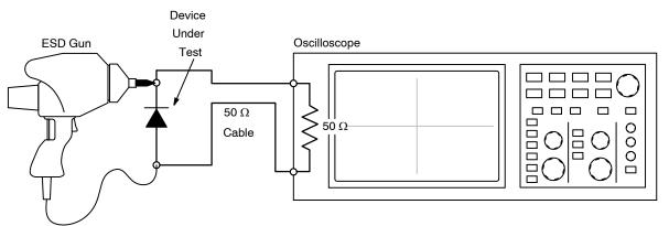
Figure 4. Diagram of ESD Test Setup
