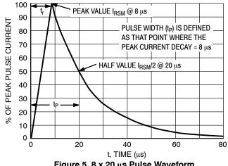
Figure 5. 8 x 20 µs Pulse Waveform
