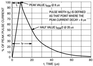
Figure 5. 8 X 20 µs Pulse Waveform
