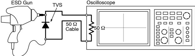
Figure 4. Diagram of ESD Test Setup
