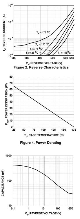
Figure 6. Capacitance vs. Reverse Voltage
