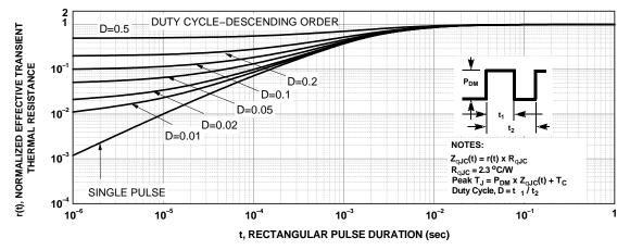
Figure 8. Junction-to-Case Transient Thermal Response Curve
