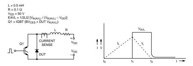
Figure 9. Unclamped Inductive Switching Test Circuit & Waveform
