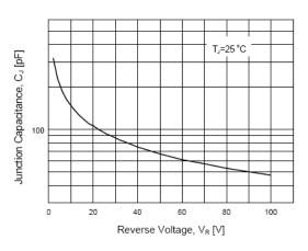
Figure 3. Typical Junction Capacitance (per diode)
