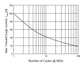
Figure 6. Non-Repetive Sureg Current (per diode)
