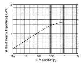
Figure 4. Thermal Impedance Characteristics (per diode)
