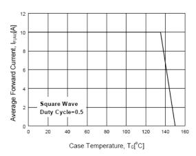
Figure 5. Forward Current Derating Curve
