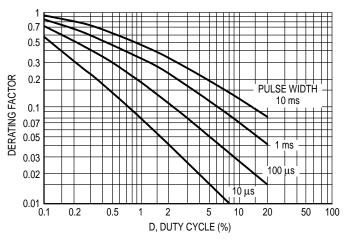
Figure 6. Typical Derating Factor for Duty Cycle
