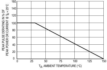
Figure 3. Pulse Derating Curve
