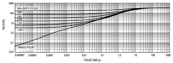
Figure 8. Thermal Response, Junction-to-Ambient (20 mm<sup>2</sup> pad)
