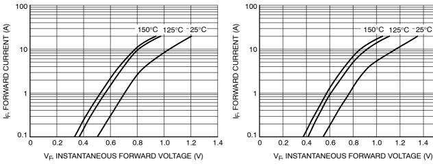
Figure 1. Typical Forward Voltage
