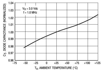
Figure 3. Diode Capacitance
