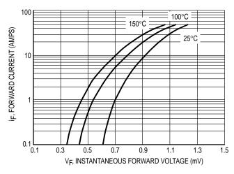
Figure 1. Typical Forward Voltage
