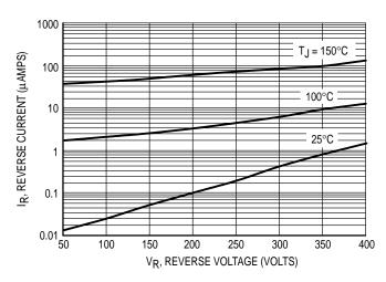
**Figure 2. Typical Reverse Current**
