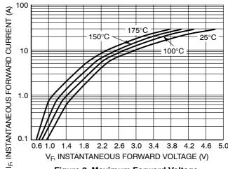
Figure 2. Maximum Forward Voltage
