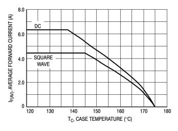
Figure 5. Current Derating, Case, Per Leg
