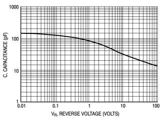
Figure 6. Typical Capacitance, Per Leg
