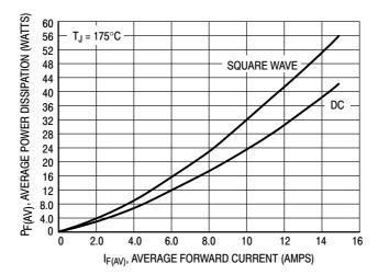
Figure 7. Power Dissipation, Per Leg
