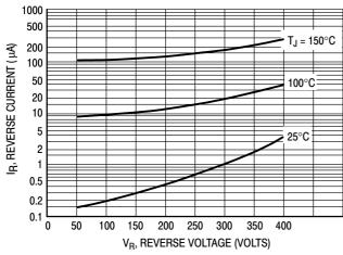
Figure 3. Typical Reverse Current, Per Leg
