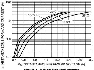
Figure 1. Typical Forward Voltage
