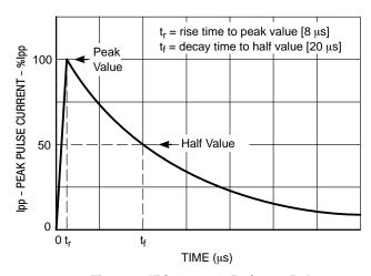
Figure 3. IEC61000-4-5 8/20 μs Pulse Waveform
