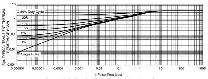
Figure 7. Typical Transient Thermal Response, Junction-to-Case
