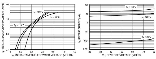
Figure 1. Typical Forward Voltage
