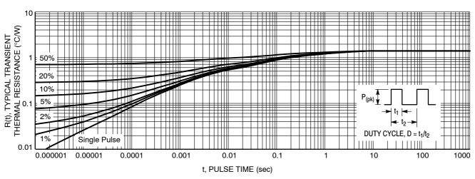
Figure 7. Typical Transient Thermal Response
