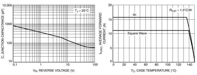
Figure 3. Typical Junction Capacitance
