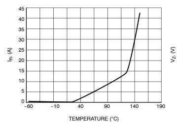
Figure 3. Typical Leakage vs. Temperature
