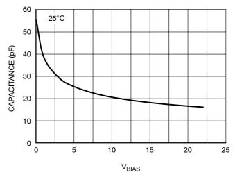
Figure 5. Capacitance vs. V<sub>BIAS</sub>
