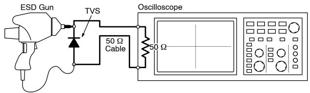
Figure 4. Diagram of ESD Test Setup
