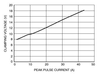
Figure 8. Clamping Voltage vs. Peak Pulse Current (8 x 20  $\mu s$  Waveform)
