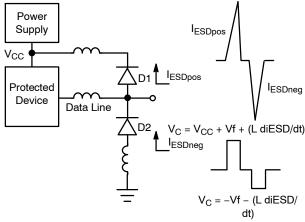
An approximation of the clamping voltage for these fast transients would be:
