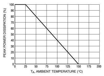
Figure 6. Pulse Derating Curve
