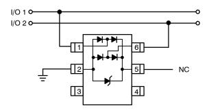
In applications lacking a positive supply reference or those cases in which a fully isolated power supply is required, the internal TVS can be used as the reference. For these applications, pin 5 is not connected. In this configuration, the steering diodes will conduct whenever the voltage on the protected line exceeds the working voltage of the TVS plus one diode drop (Vc = Vf + VTVS).
