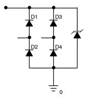
Figure 9. NUP2202W1 Equivalent Circuit
