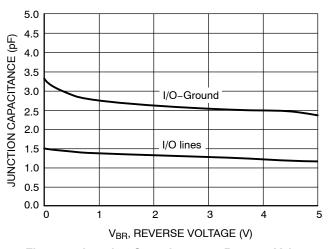
Figure 7. Junction Capacitance vs Reverse Voltage
