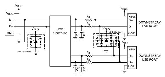
Figure 10. ESD Protection for USB Port
