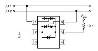
The NUP2202W1 can be isolated from the power supply by connecting a series resistor between pin 5 and  $V_{CC}$ . A 10 k $\Omega$  resistor is recommended for this application. This will maintain bias on the internal TVS and steering diodes, reducing their capacitance.
