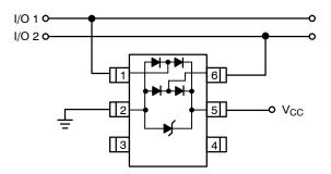
For this configuration, connect pin 5 directly to the positive supply rail ( $V_{\rm CC}$ ), the data lines are referenced to the supply voltage. The internal TVS diode prevents overvoltage on the supply rail. Biasing of the steering diodes reduces their capacitance.
