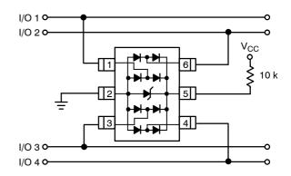
The NUP4114 can be isolated from the power supply by connecting a series resistor between pin 5 and  $V_{CC}$ . A 10 k $\Omega$  resistor is recommended for this application. This will maintain a bias on the internal TVS and steering diodes, reducing their capacitance.
