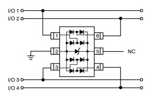
In applications lacking a positive supply reference or those cases in which a fully isolated power supply is required, the internal TVS can be used as the reference. For these applications, pin 5 is not connected. In this configuration, the steering diodes will conduct whenever the voltage on the protected line exceeds the working voltage of the TVS plus one diode drop ( $V_C = V_f + VTVS$ ).
