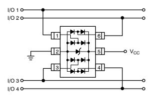
For this configuration, connect pin 5 directly to the positive supply rail ( $V_{\rm CC}$ ), the data lines are referenced to the supply voltage. The internal TVS diode prevents overvoltage on the supply rail. Biasing of the steering diodes reduces their capacitance.
