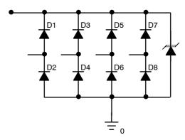
Figure 7. NUP4114 Equivalent Circuit
