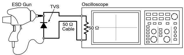
Figure 4. Diagram of ESD Test Setup
