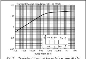
Fig.7. Transient thermal impedance; per diode;  $Z_{th j\text{-sp}} = f(t_p)$ .
