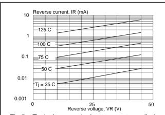
Fig.5. Typical reverse leakage current per diode;  $I_R = f(V_R)$ ; parameter  $T_j$
