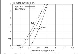
Fig.4. Typical and maximum forward characteristic  $I_F = f(V_F)$ ; parameter  $T_i$
